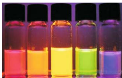
Figure 1 Emission of CdSe QDs of different size. The TOPO functionalized CdSe QDs dissolved in chloroform were excited with an UV radiation. Images were obtained in the Lin research group at the Department of Materials Science and Engineering at the Iowa State University.
